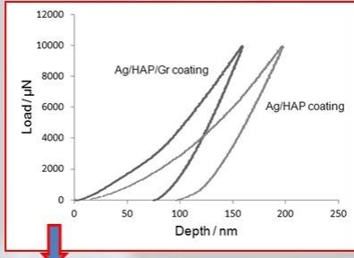
✓ Ag/HAP/Gr coating - higher hardness (lower penetration depth) and higher reduced modulus (higher slope of the initial portion of the unloading curve)
